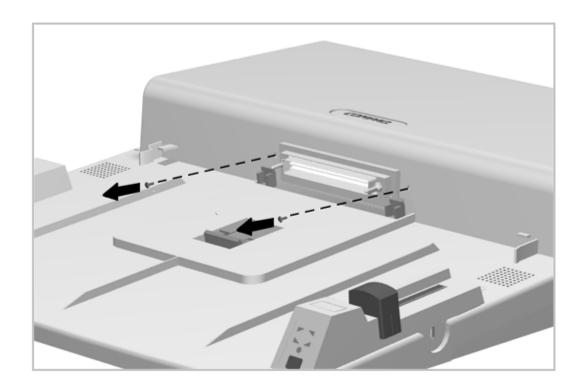
Figure 6-14. Removing the Computer Connector Screws
